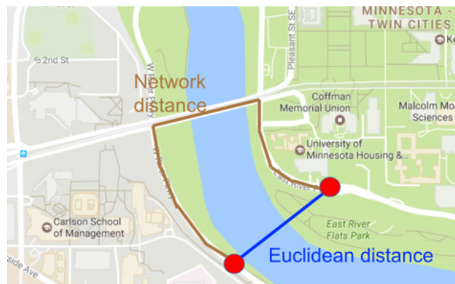
Figure 2.7: An illustrative example showing the difference between distances in Euclidean and network spaces.
